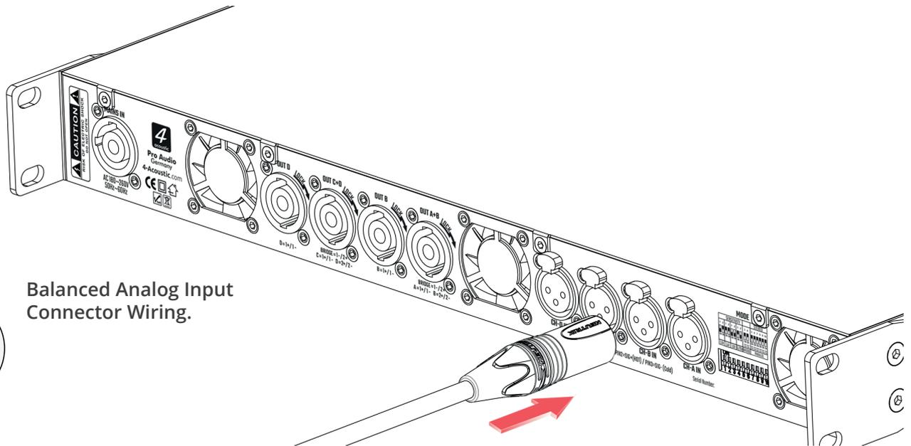
Balanced Analog Input Connector Wiring.
