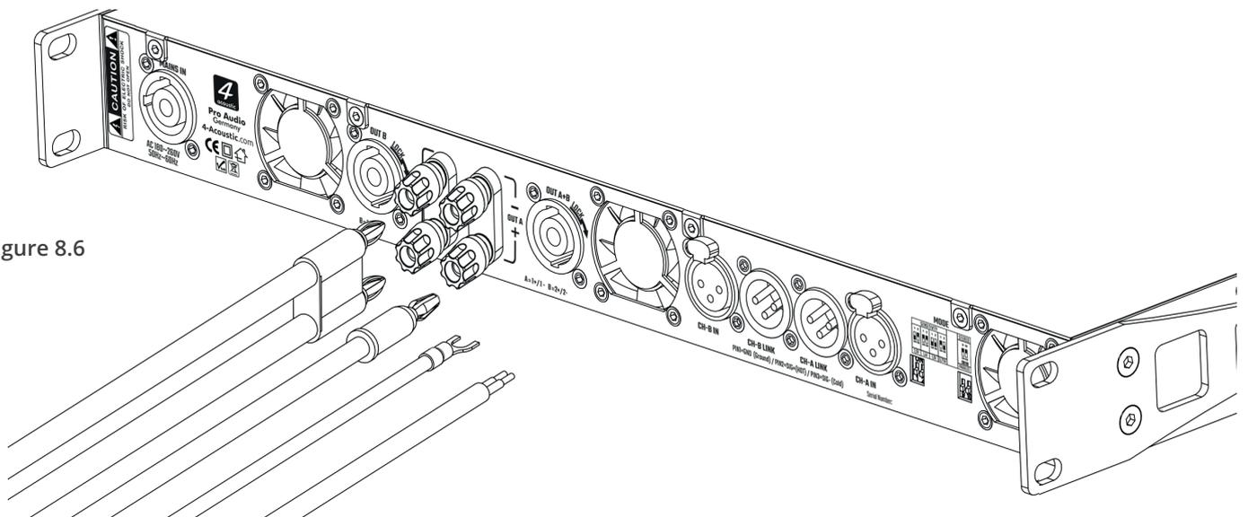
Select the appropriate size of wire based on the distance from amplifier to speaker.
