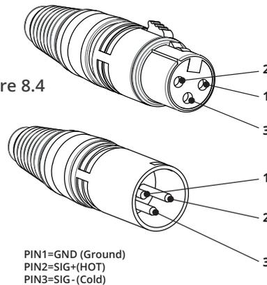
Unbalanced Analog Input Connector Wiring
